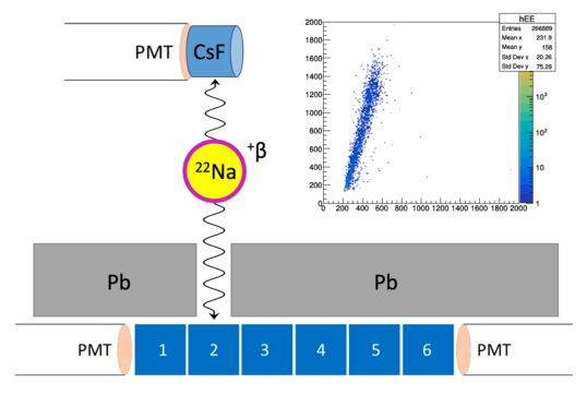
**Fig. 1**. Sketch of the CsF and pseudo-bar placement during the timing characterization experiments. The placement of the stop CsF detector is not shown here. The histogram inset shows the energy spectrum from both PMTs,  $E_{left}$  vs  $E_{right}$ , with  $\gamma$ -rays only being exposed to crystal-2 as shown in the diagram. Units in the inset histogram are ADC channel.
